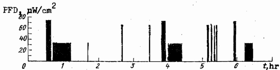
Figure 1. First Type of Irradiation Characterized by Intermittence of Each Parameter -- Intensity, Period of Irradiation, and Intervals Between Irradiation
