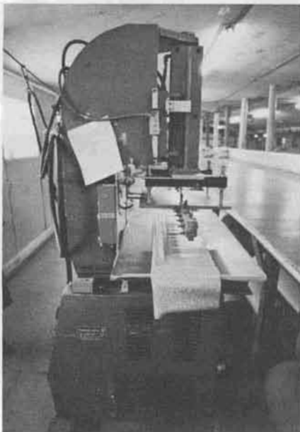
Figure 4 RF sealer (included into shuttle-tray type). The operators (two) stand in front of the device.
