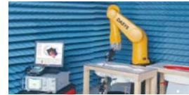
Figure 1. Robotic arm with electric field probe for SAM (Source: Speag DASY 52 Info Sheet)
