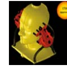
Figure 2. SAM Uniform Phantom Source: Speag Phantom Product Flyer CTIA is Cellular Telecommunications Industry
